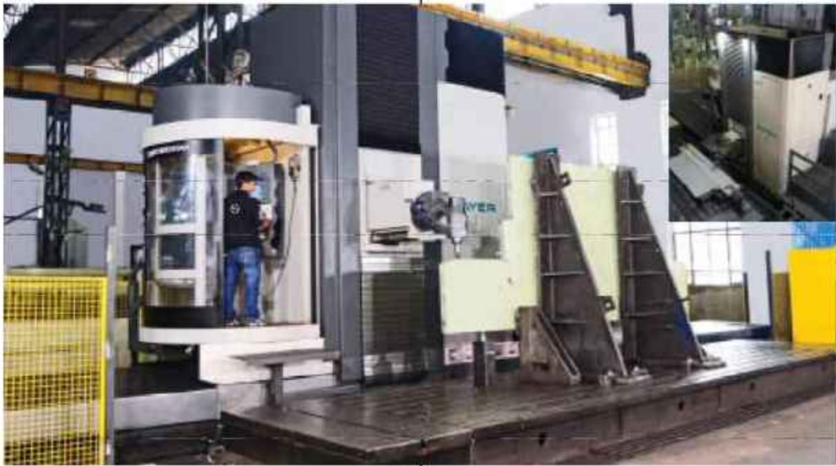
SINGLE SETUP MOVING COLUMN HORIZONTAL & VERTICAL CNC MILLING MACHINE
