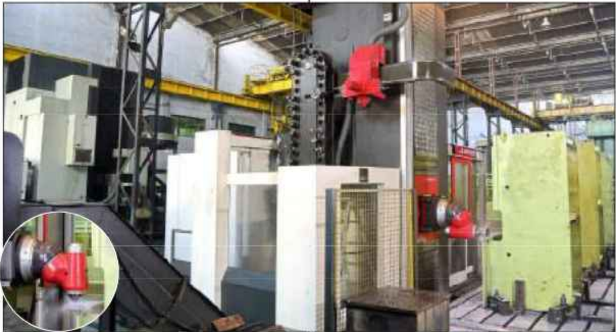
SWASTI FLOOR BORING MACHINE IS THE BEST MACHINE FOR MILLING AND DRILLING, CAPABLE OF HANDLING UP TO 9 METERS FRAMES IN SINGLE SET-UP WITH SPINDLE ROTATION AT 500 AND AUTOMATIC TOOL CHANGER (ATC)
