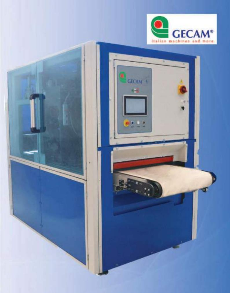
Machines designed for deburring, finishing and rounding edge of metal surfaces with useful working width from 300 mm up to 1350 mm
