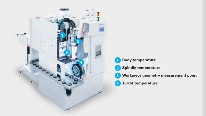
A very normal process for many – machines undergo a warm-up process before starting production. This uses relatively large quantities of energy – with zero output.
