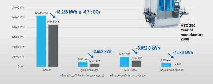
This example focuses on a VTC 250 shaft turning machine dating from 2008 – in good condition with no leaks or similar defects. The energy flow diagram highlights three areas in which the machine is no longer state of the art, namely the hydraulic unit, cutting fluid pump and cooling unit. All three units were replaced. As a result, the user saves around 18,000 kWh per annum or around 6.7 tonnes of  $\rm{CO}_2$ . This is more than the consumption of two single-family houses per year.
