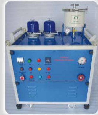
Hydraulic Oil Cleaning System
