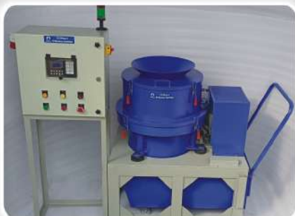
Oil Recovery Centrifuge (Automatic)
