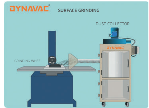
Dust Collection from surface grinding Operation
