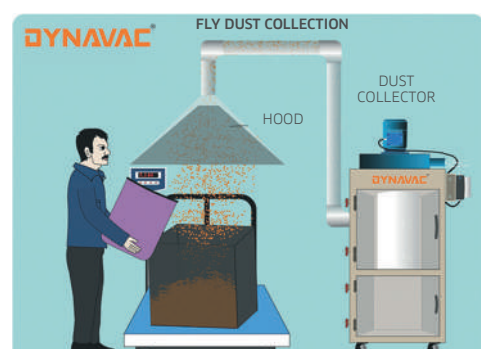
Fly dust collection during product weighing with fixed canopy hood
